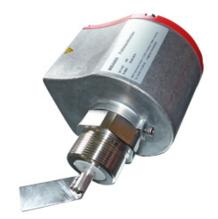
Direct drive without gearbox, powerful motor with miniature paddle, selectable pre-set parameter combinations for universal use – those are the main features of the new MBA800 rotating paddle series for level measurement. The adjustment of the different motor control parameters can be adapted for different types of bulk goods and their behaviour in the respective application.
